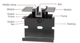
Under no circumstances should the clamp touch the glass or deform the frame. Be sure to avoid shadowing effect from the pressure clamp.
