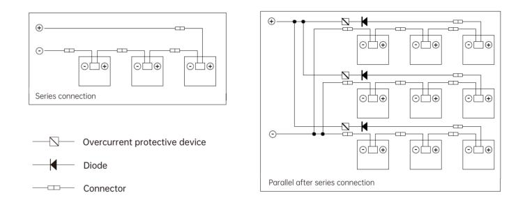
If there has reverse current exceeding the maximum fuse current flowing through the module, use overcurrent protection device with the same specifications to protect the module. If more than two strings are connected in parallel, there must be an overcurrent protection device on each strings of module.
