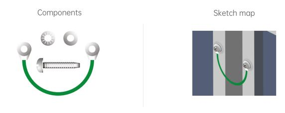
We recommend using the following method to ground correctly, as shown in the figure.
