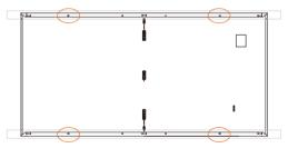
The beam perpendicular to the short frame
