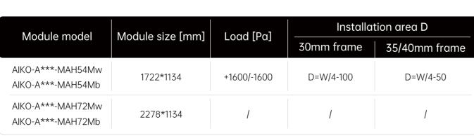
Table 4: Single glass modules clamp mounting diagram and corresponding loads, short frame (B)
