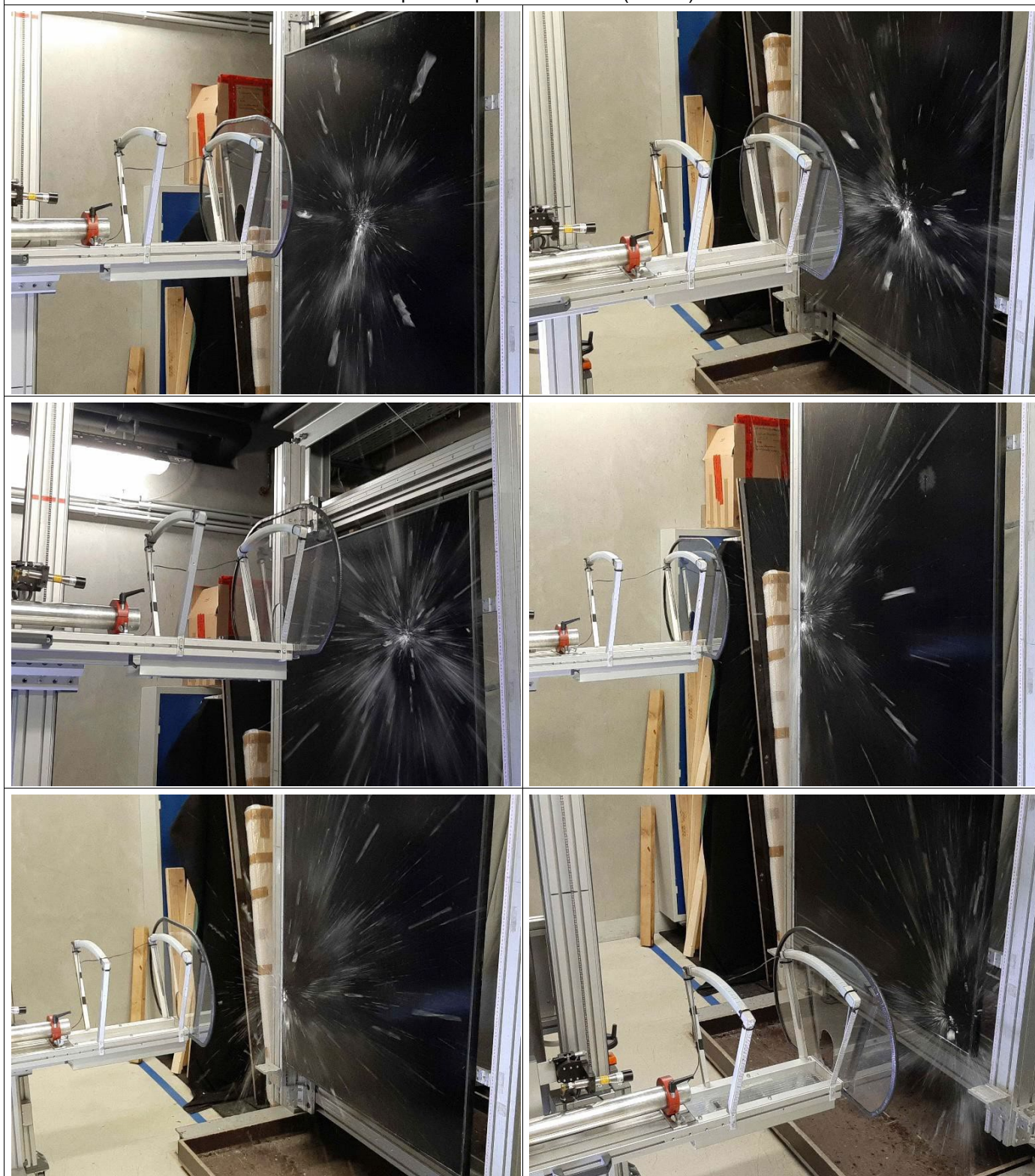
Example of Impacts on Module (40 mm)
